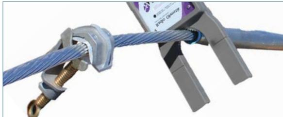
The Ohm Check generates an AC Current, allowing utility personnel to measure resistance on de-energized lines with the Ohmstik for an immediate verification of splice condition.
